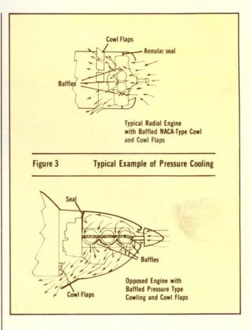
baffles all have attached rubber seals to aid in properly sealing the pressure area from the lower and aft areas.
